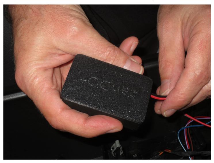
Finally, connect the other end of the red & black connector assembly into canDO+
